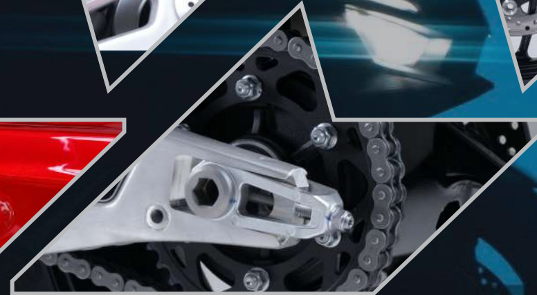
Quick-release Rear Wheel Design
